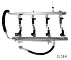
The Siemens fuel injection values are the dual outlet "directional angle plate" type with a *coil reisistance of approximately 12 ohms each.*
